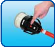
Press the red switch to turn on LED illuminates green Flash at slow rate indicates normal STANDBY mode.
